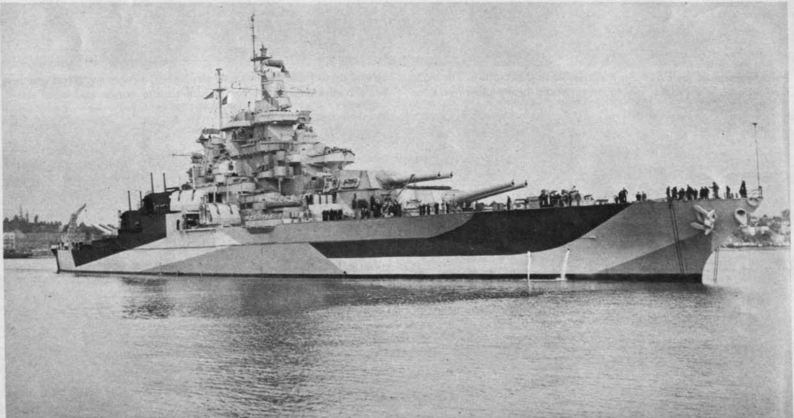
Dual-purpose mounts , four on each side, provide West Virginia with modern AA protection. Similarity to the refitted Tennessee in this and
